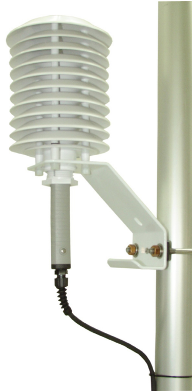
FIGURE 1. HMP45C and 41003-5 Radiation Shield on a Tripod Mast
